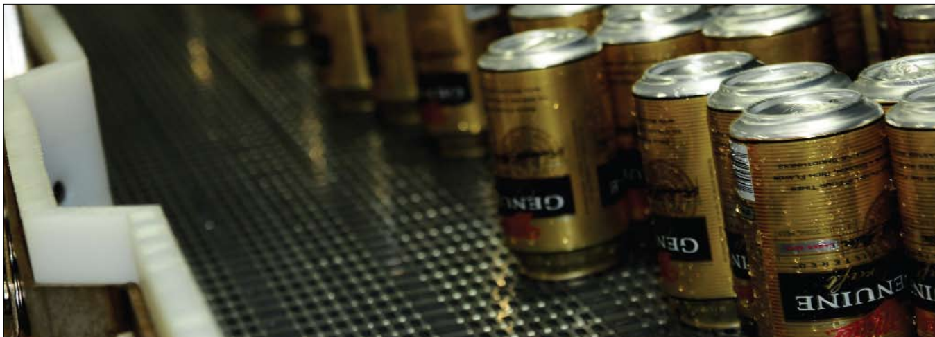
Cans of Miller Genuine Draft enter the heat-pasteurizing tunnel where impurities are eliminated and freshness ensured.
