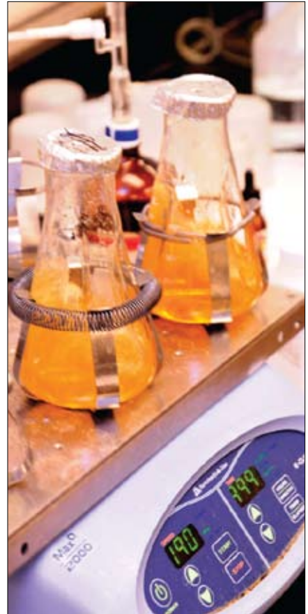
Beer samples are agitated prior to testing to remove carbonation and ensure uniformity.
